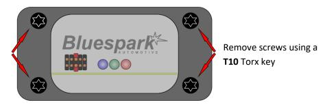
To increase performance move the red jumper to an alternative pin set to the right. To decrease performance or if the current state of tune has **caused an engine management light** to appear when driving) move the jumper to an alternative pin set to the left until the problem is resolved. Starting problems are down to a connection issue as the box setting does not affect engine idle.
