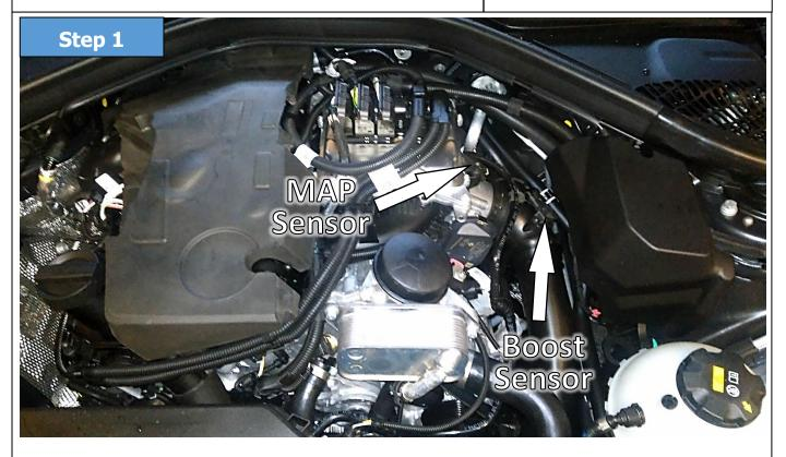
• Remove the engine cover, it should come off with a firm tug.
