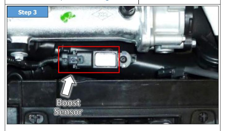
Unplug the Boost Sensor connector (3 pin) by pressing down the releasing clip and pulling back the connector.
