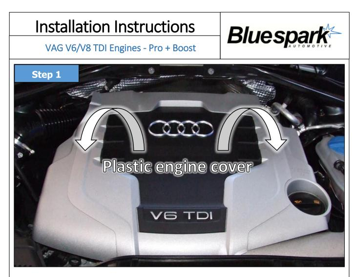
• Remove the plastic engine cover by lifting it off the engine, then the engine should look similar to the photo in Step 2.
